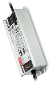
The HLG-60 series is a 60W AC/DC LED driver featuring dual mode constant current and constant voltage output. Operating at 90.5% efficiency, the driver is able to operate in environments ranging in temperatures from -40°to +90°. Its high IP67 ingress protection rating allows to it operate comfortably in outdoor and indoor applications. The reliable Mean well driver comfortably drives the flood light to achieving the rated 50 000 hour life span.
